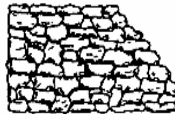
View 2. Coursed rubble masonry
